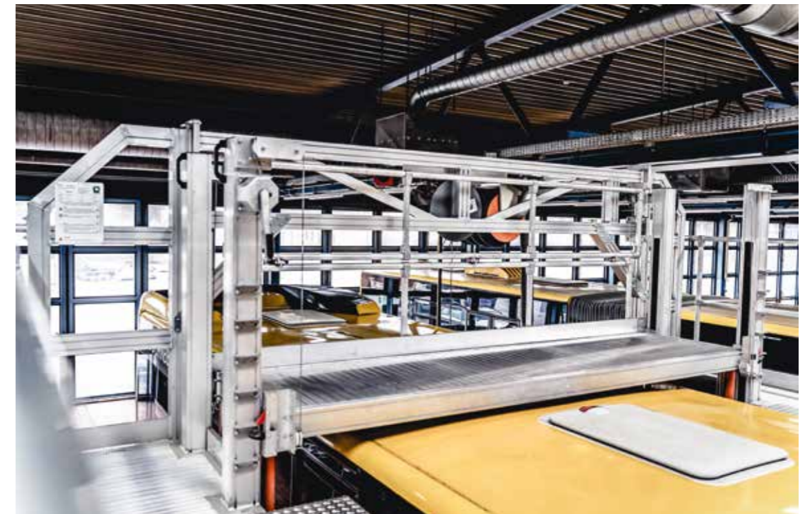
The height of the front work platform can also be adjusted. It serves both as a bridging step and as a work surface
