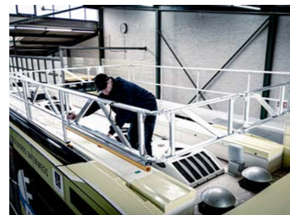
Side protective cage for securing the work area, optionally with lowerable skirting boards
