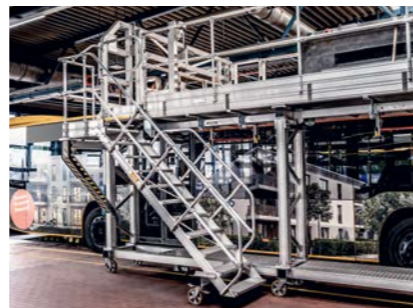
Stairs with handrail and railing as well as self-closing safety door
