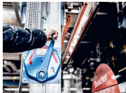
Platform widening by cable winch
