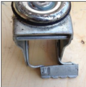
Foot pedal distortion as a result of a significant frontal impact; it is likely the top plate and bearing will be distorted as well.
