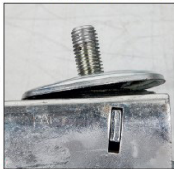
Mounting plate distortion as a result of a single significant impact or multiple lower level impacts. Even if the rest of the castor is in good condition, it must be replaced.
