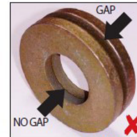
DO NOT FIT DISC SPRINGS LIKE THIS
